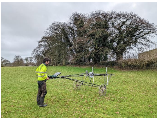
Bartington Grad 601-2 mounted on Bartington Cart system
