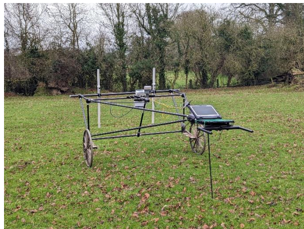
Bartington Grad 601-2 mounted on Bartington Cart system
